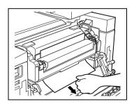
5 Move the two lock release levers for the oil-coating unit in the direction of the arrows.
